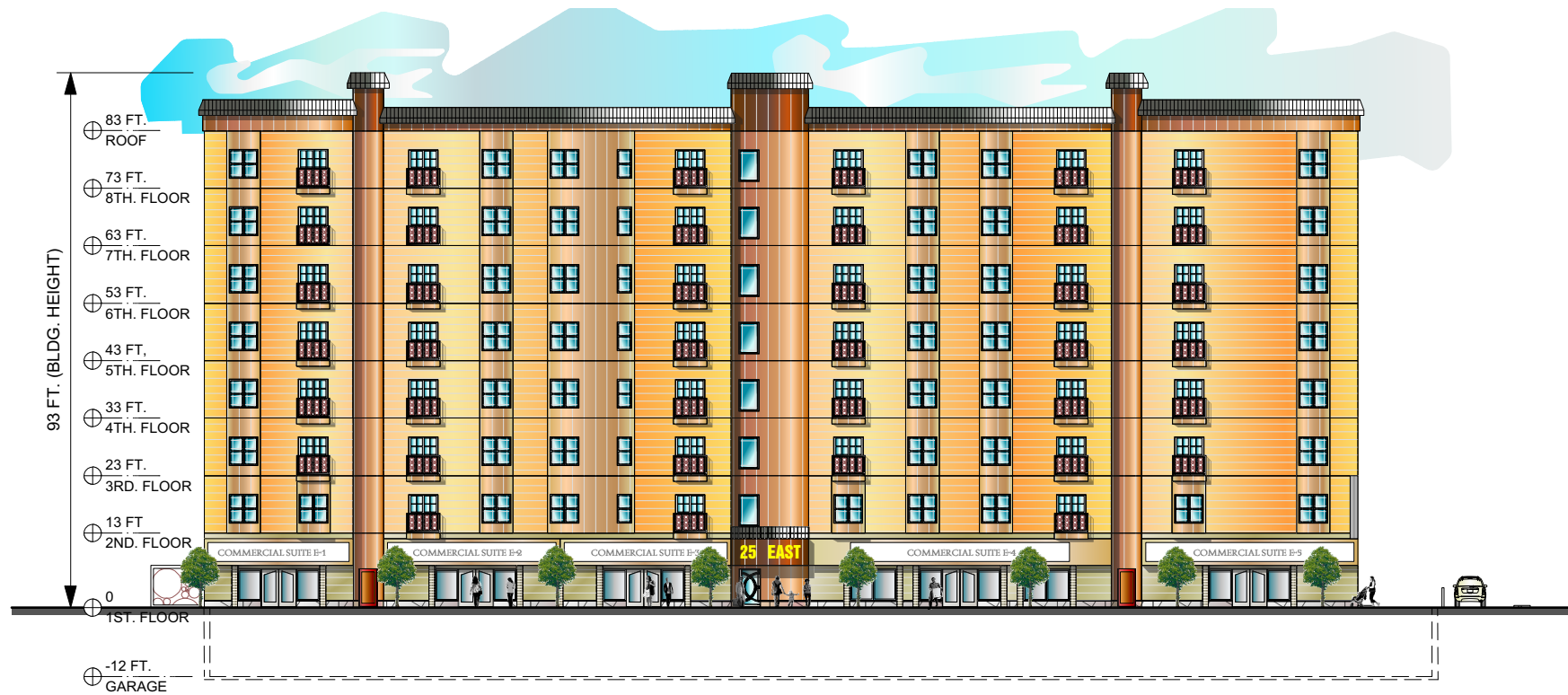
○ FRONT ELEVATION (23RD STREET) Scale: 1" = 30 ft
