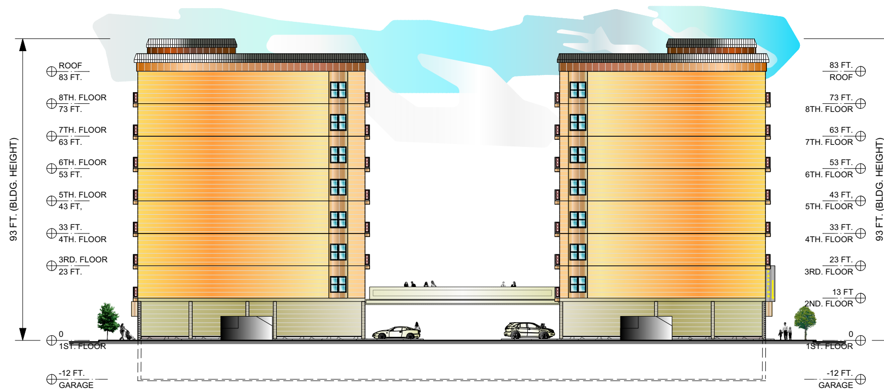
LEFT SIDE ELEVATION (SERVICE AREA) Scale: 1" = 30 ft
